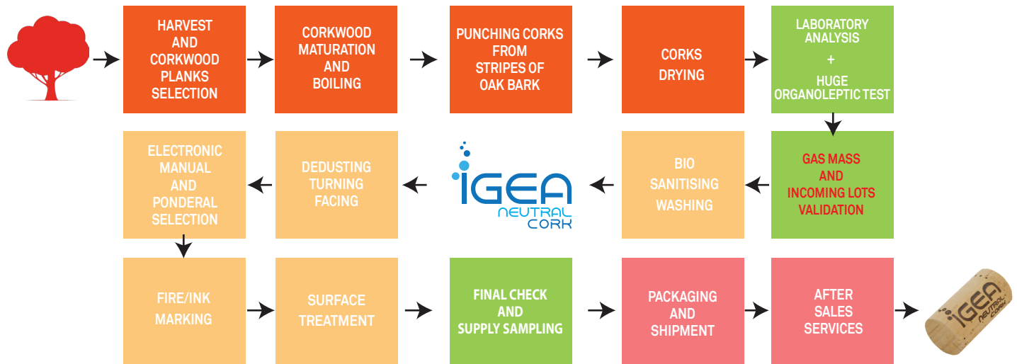
process stages for IGEA Neutral Cork stoppers
